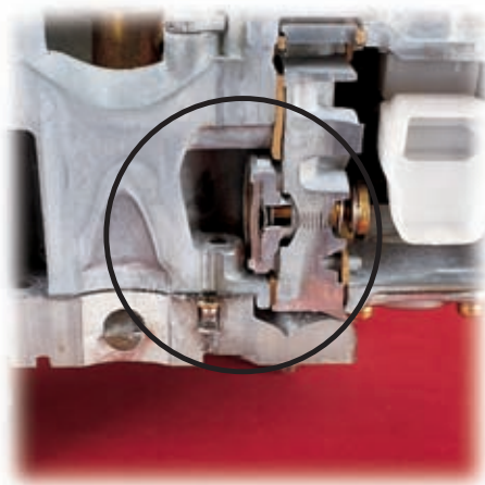
Cut-away of power valve blow-out protection.
